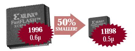
by John Ahn, CPLD Product Manager, john.ahn@xilinx.com The FastFLASH family of CPLDs just got better with the recent introduction of the XC95144. This newest member of the XC9500 family completes the fastest growing line of CPLDs in the industry. The XC95144 features 144 macrocells with 7.5 ns pin-to-pin delays and is offered in 100-pin TQFP, 100-pin PQFP, and 160-pin PQFP packages.
