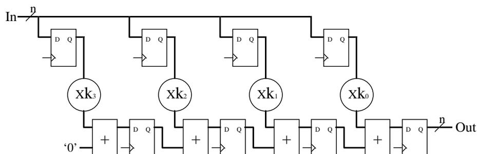
**Fig 3. 'Inverse' FIR structure employing cascaded pipelined adders**
