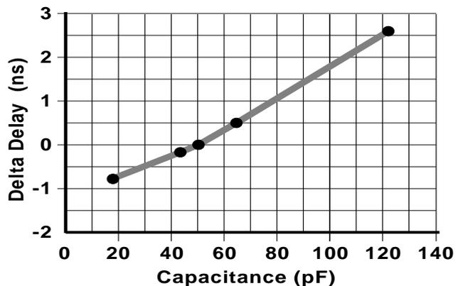
**Figure 1: Delay Factor at Various Capacitive Loads**
