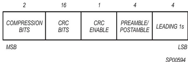
Figure 12: 27-bit Header
