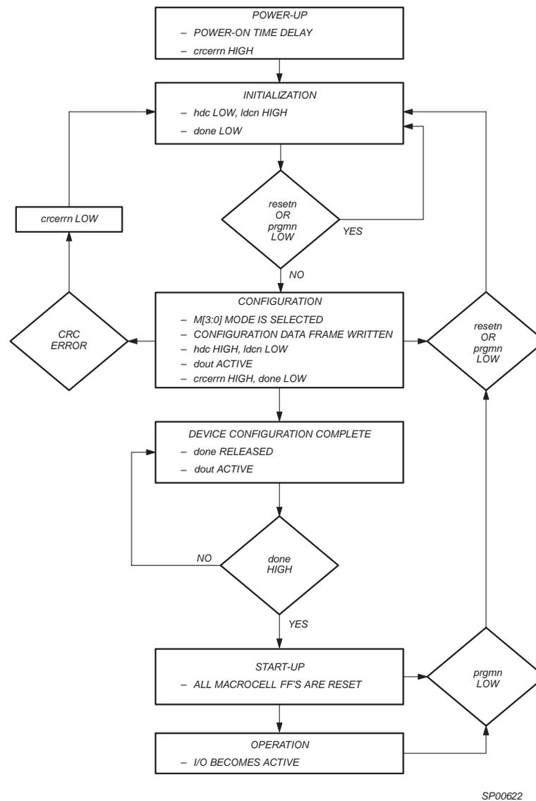
Figure 8: Chart Of Initialization, Configuration, and Operating States
