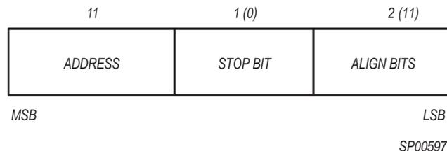
Figure 14: Compressed Frame
