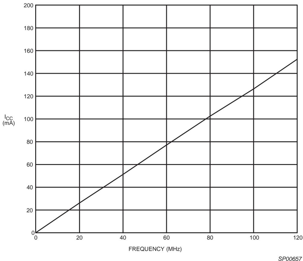
**Figure 6:**  $I_{CC}$  vs. Frequency at  $V_{CC} = 3.3V$ , 25°C
