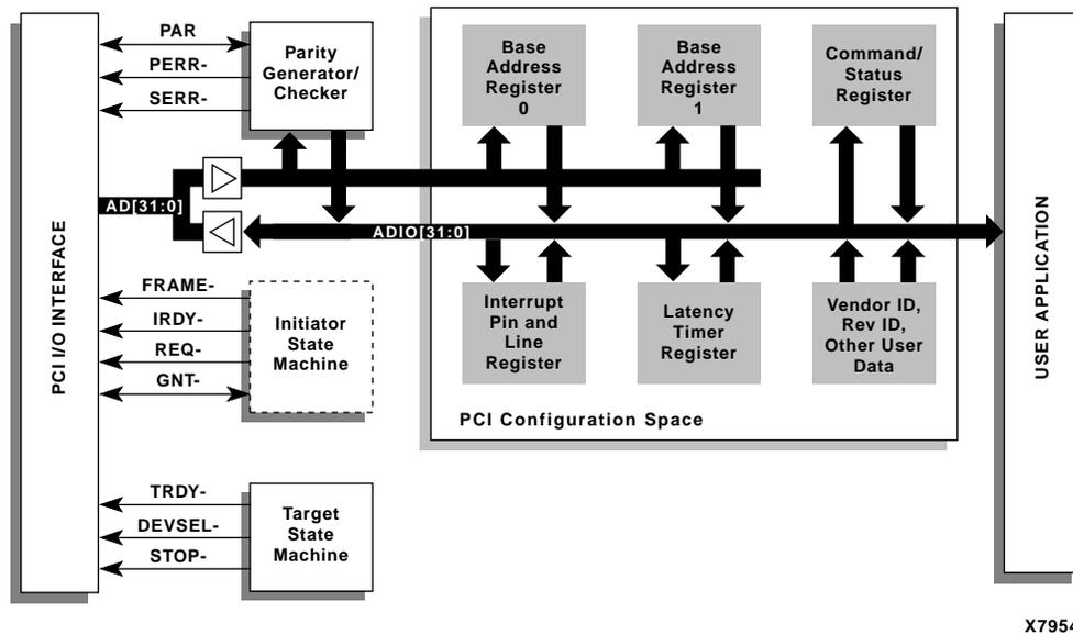
Figure 1: LogiCORE PCI32 SpartanXL Interface Block Diagram (one BAR only in XCS20XL)
