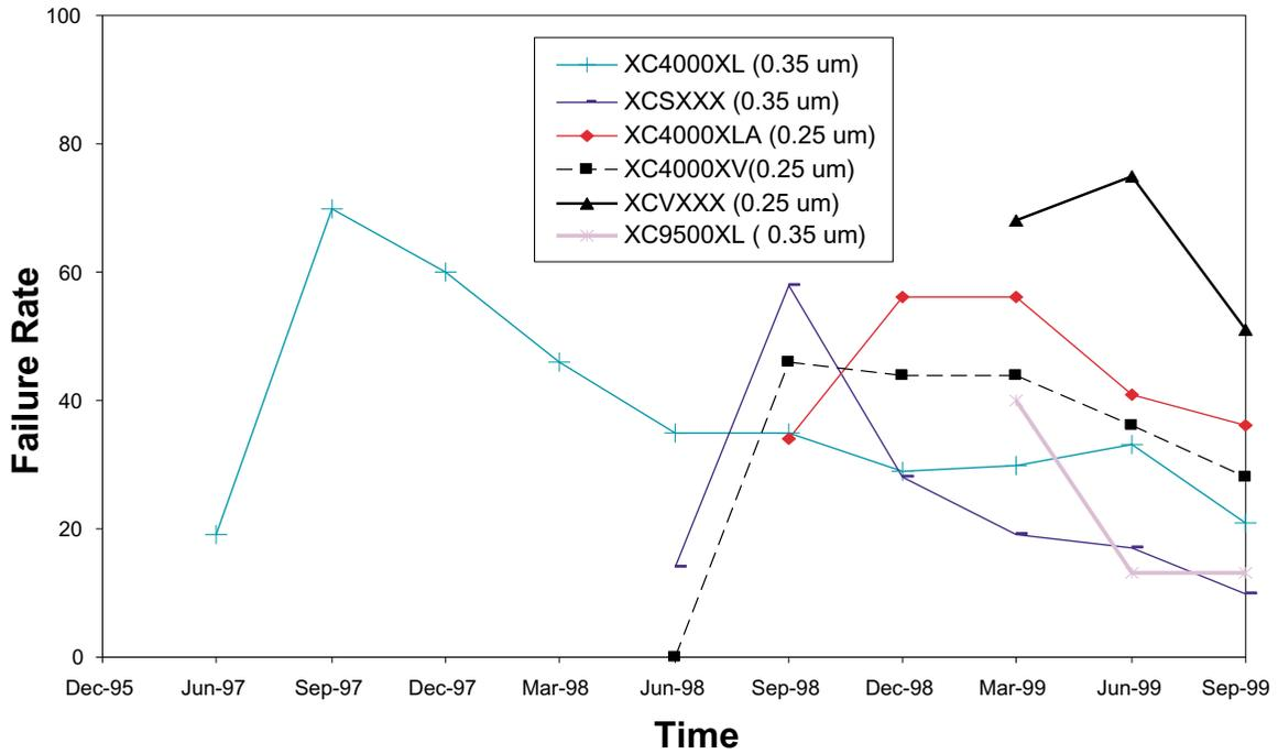
Figure 2: Failure Rate in FITS at Tj = 55°C for New Products-XSJ
