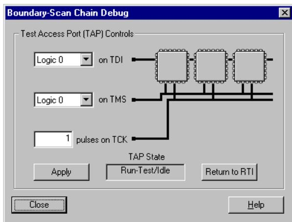
**Figure 5: Boundary-Scan Chain Debug**
