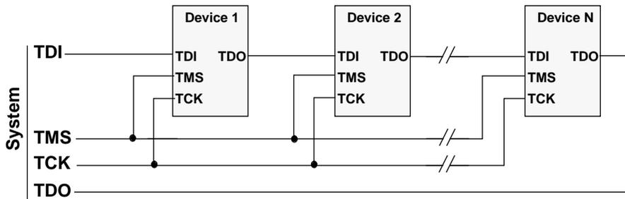
Figure 4: Single Port Serial Boundary-Scan Chain
