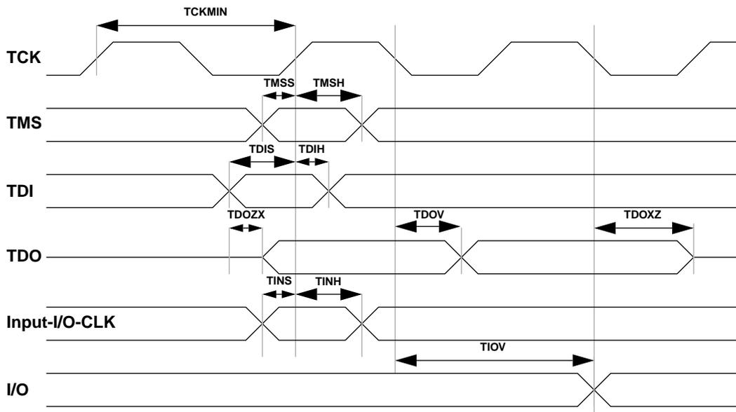
Figure 1: Test Access Port Timing
