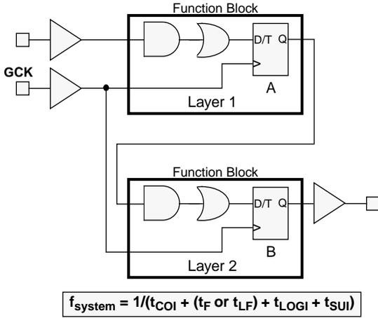
Figure 7: Multiple Flip-Flops with Single Level Logic (Note: Global Clock)
