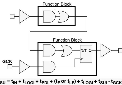
Figure 6: Flip-Flop with Multiple-Pass Logic
