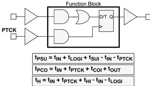
Figure 8: Single Flip-Flop with Product Term Clock
