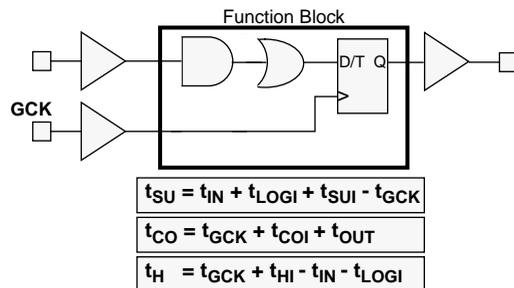
Figure 5: Simple Flip-Flop Path
