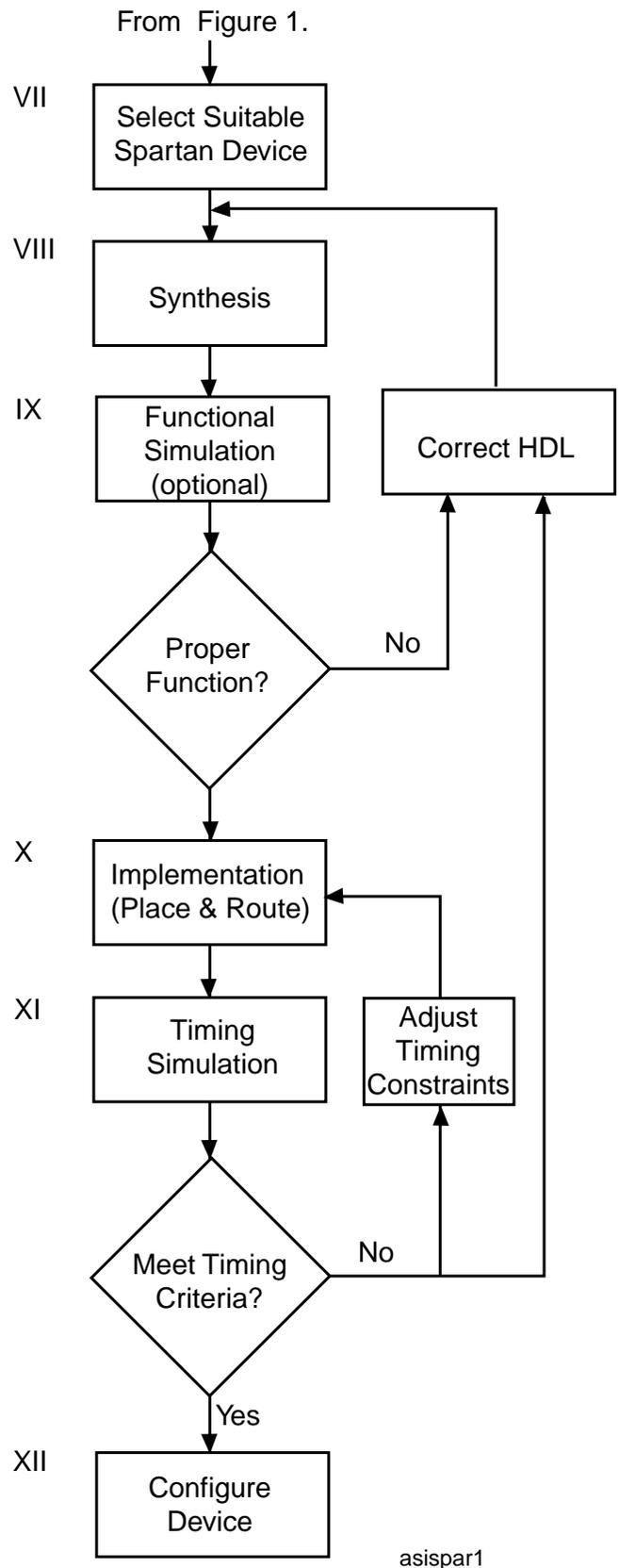
Figure 2: Synthesis-Implementation Flow
