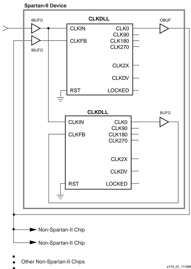
**Figure 10: DLL Deskew of Board Level Clock Between Spartan-II and Multiple Non-Spartan-II Devices**
