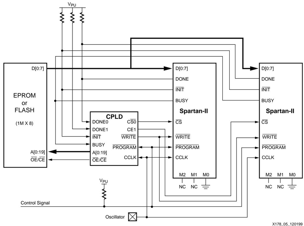
Figure 5: Connecting Multiple FPGAs for Parallel Configuration Chain
