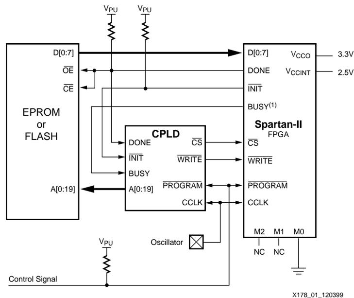
**Figure 1: Slave Parallel and EPROM Interface Circuit Diagram**
