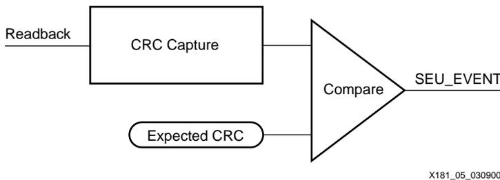
Figure 5: Readback CRCComparator
