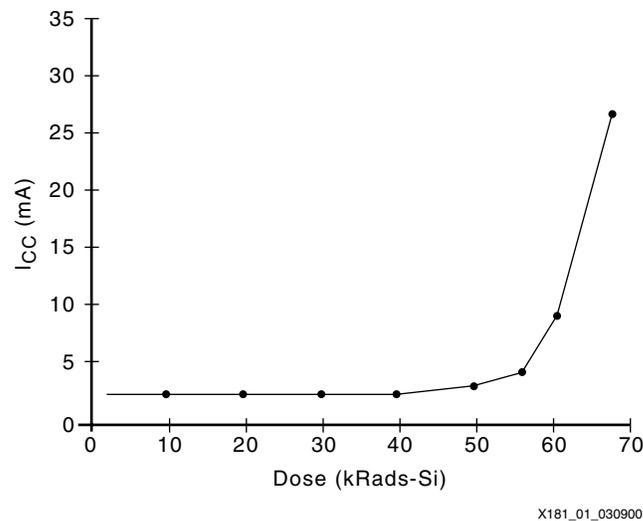
Figure 1: I<sub>CC</sub> (mA) vs. Total Dose (KRads)
