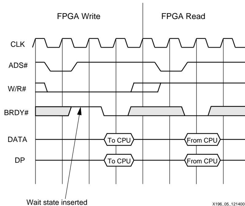
Figure 5: Non-pipelined Read and Write with Wait States
