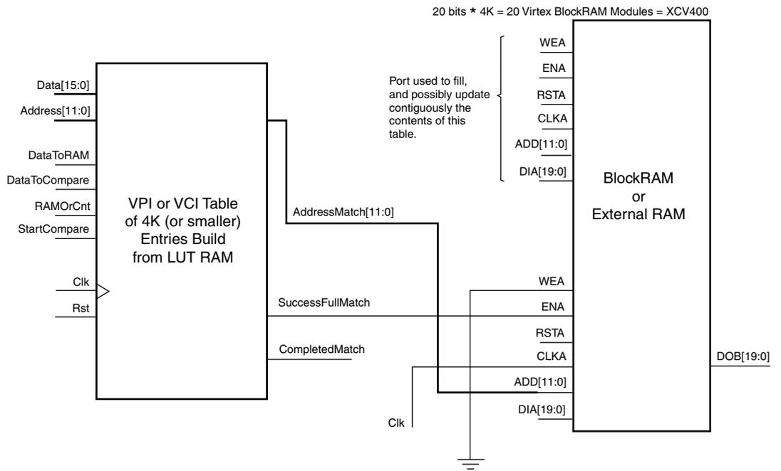
Figure 10: Complete CAM Solution
