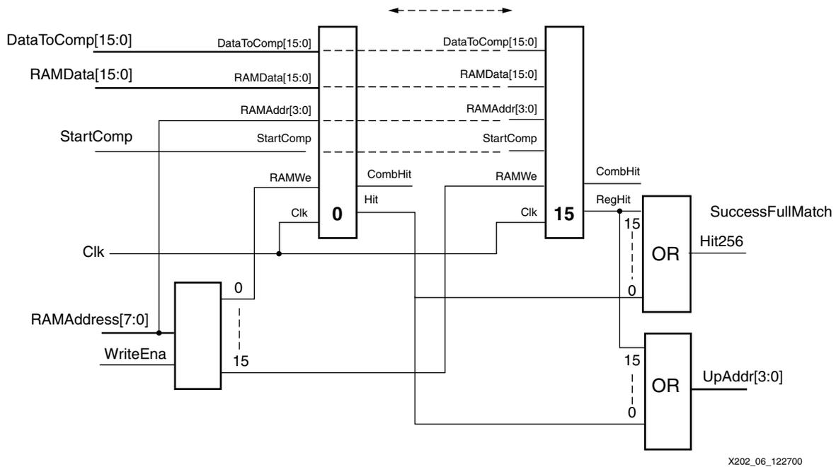
Figure 6: EntriesEngine256 CAM
