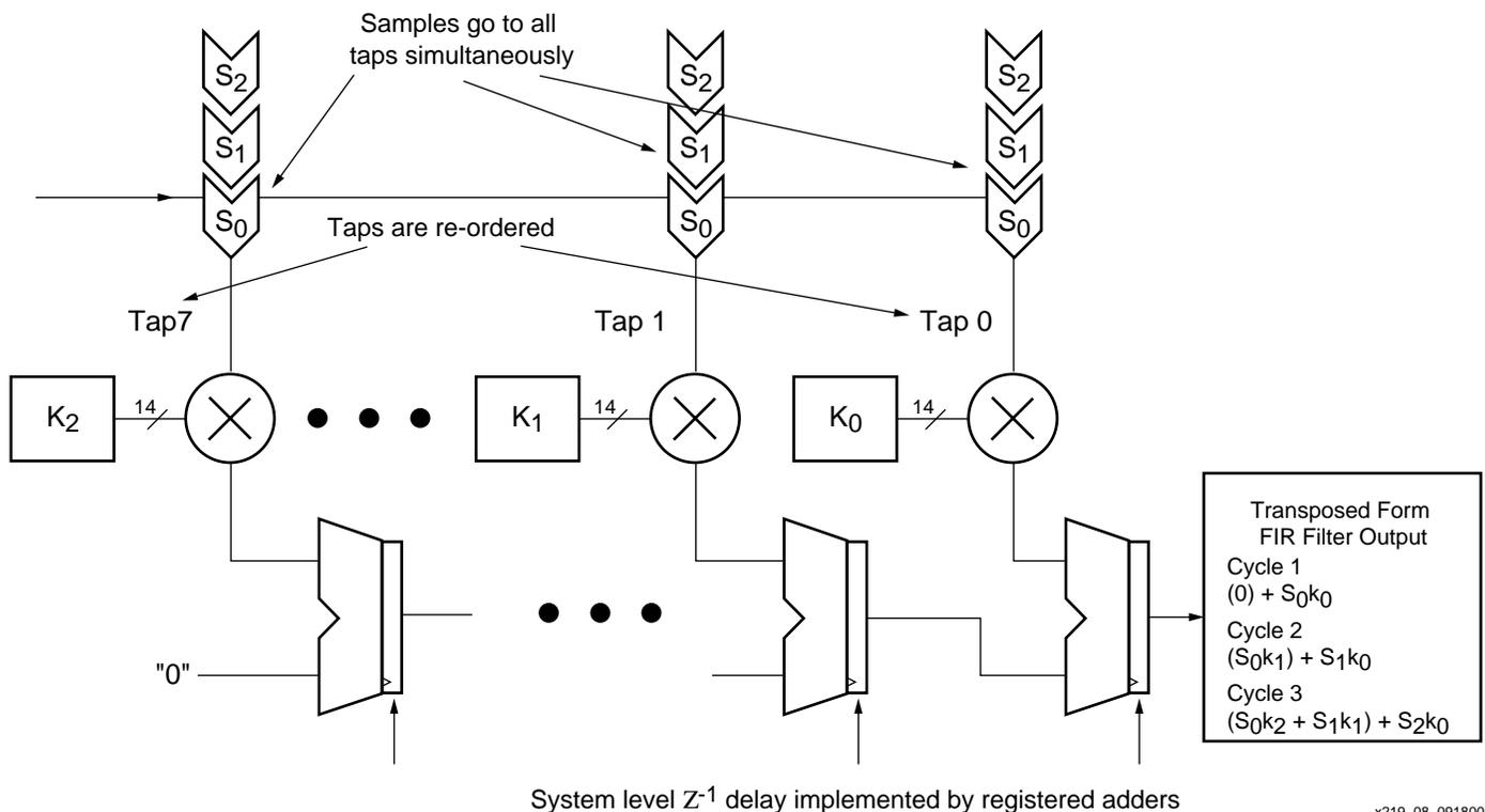
Figure 8: Transposed Form FIR Filter Block Diagram
