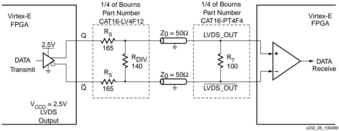
Figure 5: Virtex-E LVDS Line Driver and Receiver Schematic.
