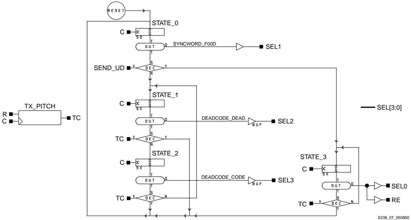
Figure 7: RE\_CTL State Machine Schematic
