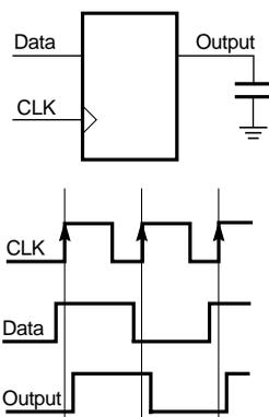
**Figure 1: Clocked Output**
