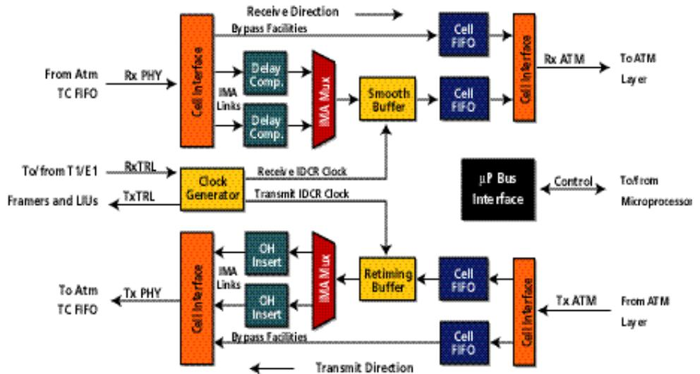
Figure 4 - Functional block diagram.
