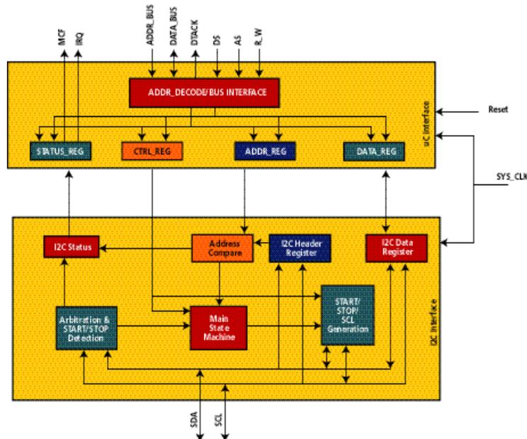
Figure 2 - CoolRunner I²C Controller block diagram.
