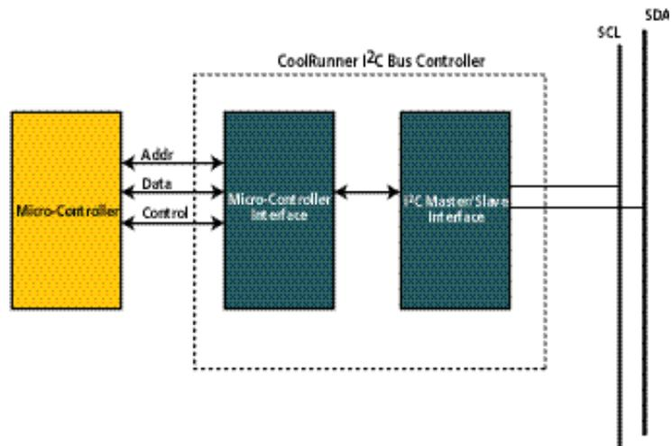
Figure 1 - CoolRunner I<sup>2</sup>C Bus Controller.
