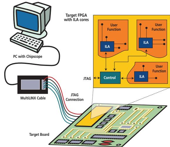
Figure 2 - Integrated logic analysis.
