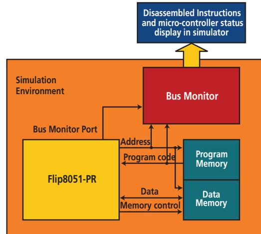
Figure 3 - Typical use of the Bus Monitor functionality.
