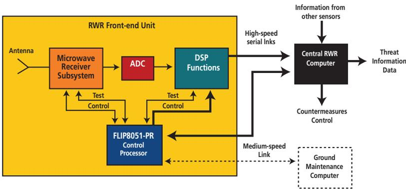
Figure 1 - Radar Warning Receiver (RWR) system.
