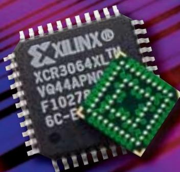
Coolrunner CPLDs can be used to implement various functions within Smart Card Readers, and are especially beneficial in handheld, lightweight, battery-powered applications.
