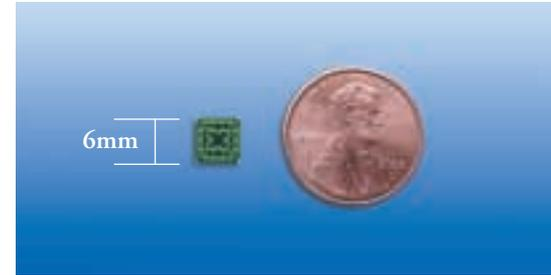
Figure 2 - CoolRunner XPLA3 64-macrocell 56-pin, 0.5mm pitch Chip Scale package.
