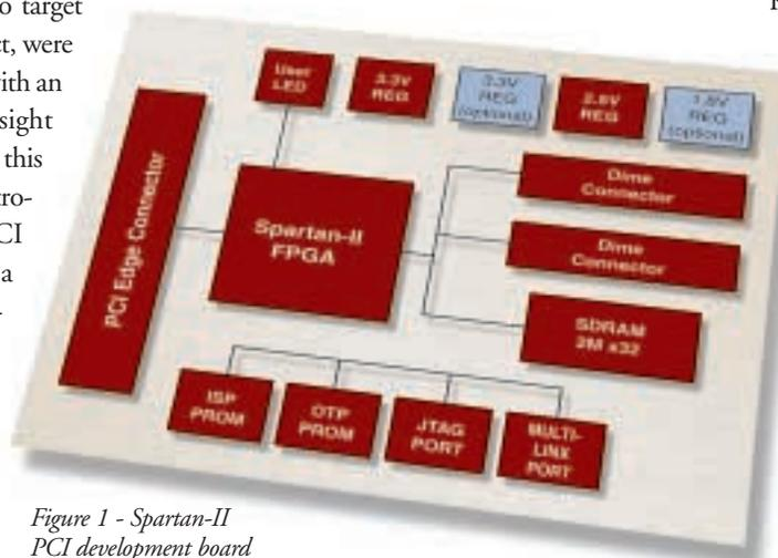
Figure 1 - Spartan-II PCI development board
