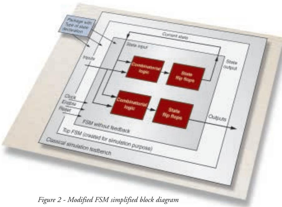
Figure 2 - Modified FSM simplified block diagram
