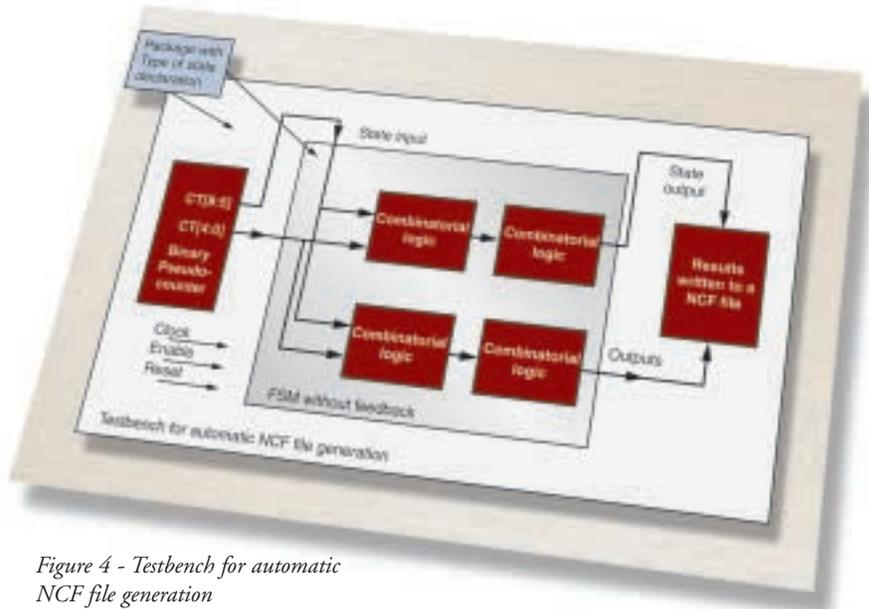
Figure 4 - Testbench for automatic NCF file generation
