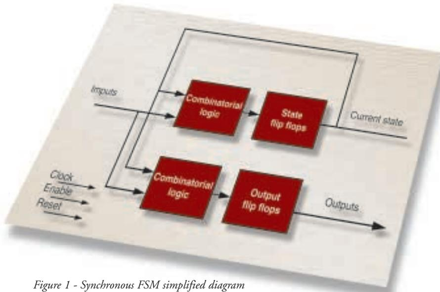
Figure 1 - Synchronous FSM simplified diagram
