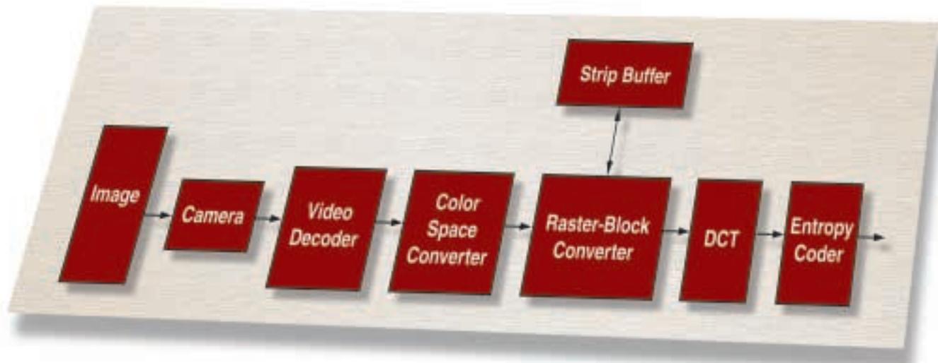
Figure 1 - LogiCOREs in a typical digital video/image processing chain
