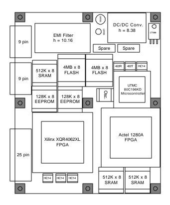
Figure 2 AIM Preliminary Flight Board Layout
