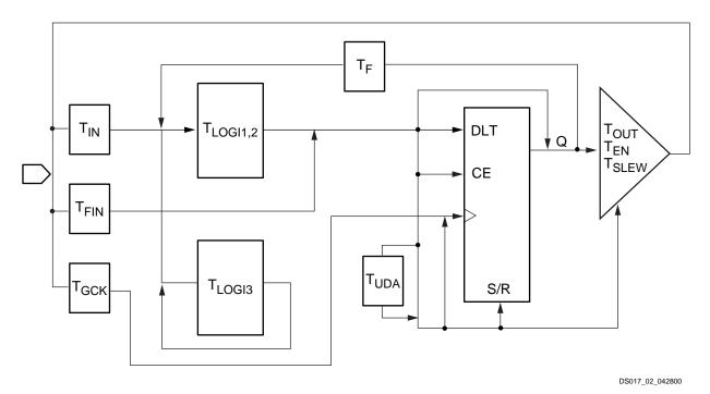
Figure 7: XPLA3 Timing Model
