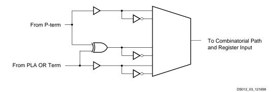
Figure 4: Variable Function Multiplexer
