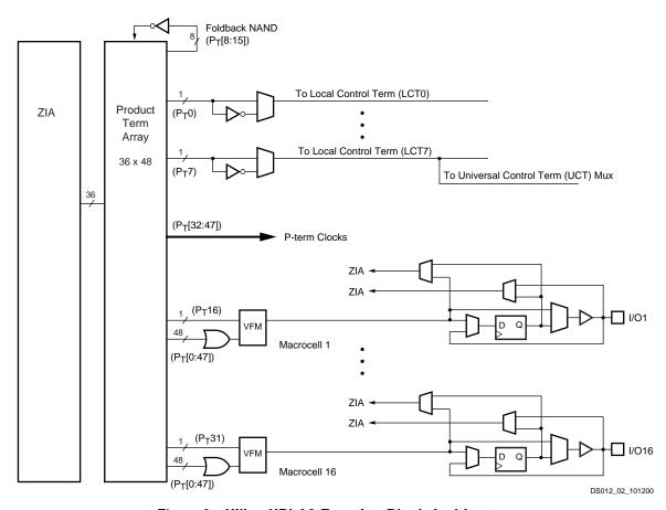
Figure 3: Xilinx XPLA3 Function Block Architecture
