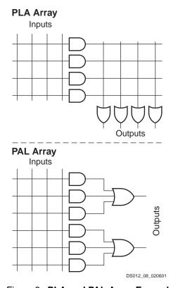
Figure 2: PLA and PAL Array Example
