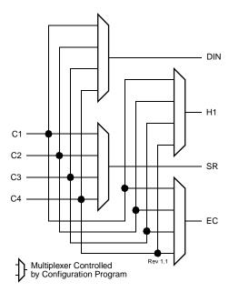
Figure 4: CLB Control Signal Interface
