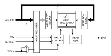
Figure 12: Logic Diagram for the Single-Port RAM
