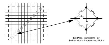
Figure 10: Programmable Switch Matrix
