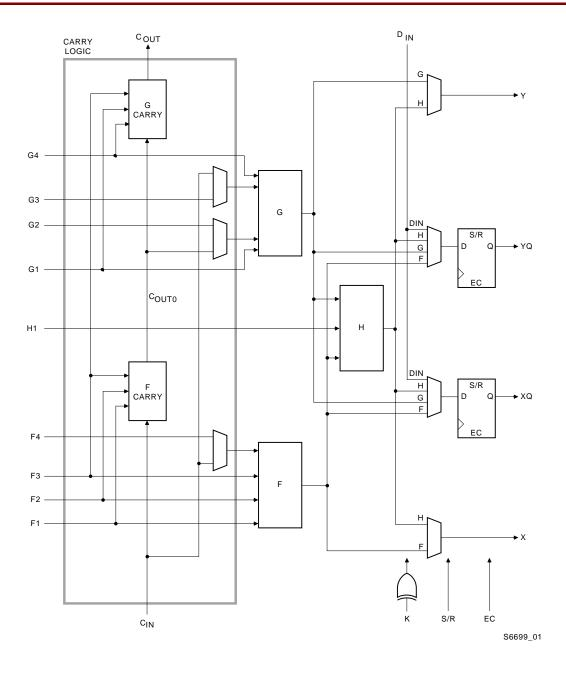
Figure 16: Fast Carry Logic in Spartan/XL CLB
