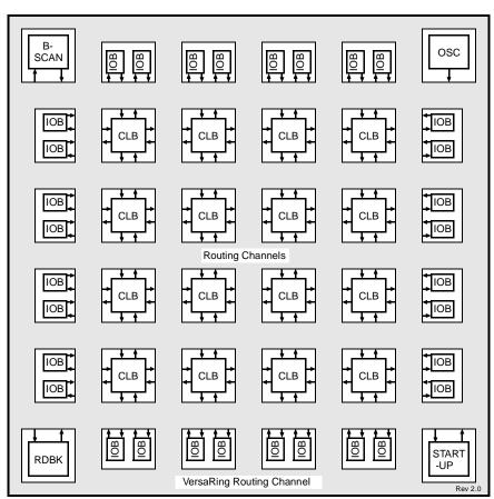
Figure 1: Basic FPGA Block Diagram
