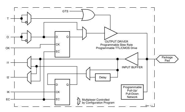
Figure 5: Simplified Spartan/XL IOB Block Diagram
