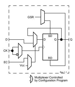
Figure 6: IOB Flip-Flop/Latch Functional Block Diagram
