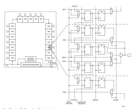
Figure 20: Spartan/XL Boundary Scan Logic
