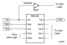
Figure 22: Boundary Scan Schematic Example
