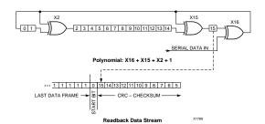
Figure 29: Circuit for Generating CRC-16
