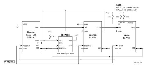
Figure 25: Master/Slave Serial Mode Circuit Diagram
