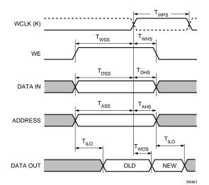
Figure 13: Data Write and Access Timing for RAM
