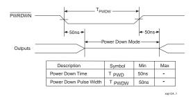
Figure 23: PWRDWN Pulse Timing
