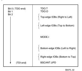
Figure 21: Boundary Scan Bit Sequence
