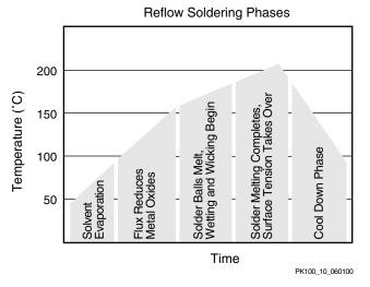
Figure 10: Soldering Sequence
