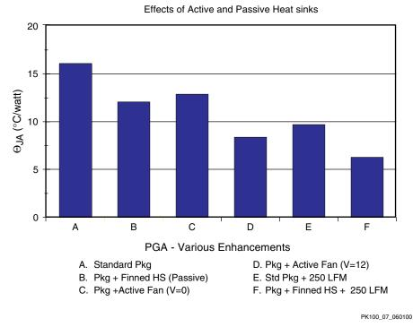
*Figure 7:* **PGA Thermal Data** (Effects of Active and Passive Heat Sinks)
