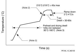
Figure 13: Typical Conditions for Vapor Phase Reflow Soldering
