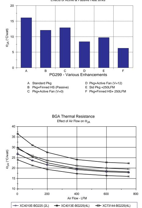
PG299 Thermal Resistance Effects of Active & Passive Heat sinks
