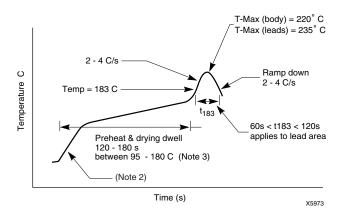
Figure 6: Typical Conditions for IR Reflow Soldering
