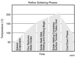
Figure 4: Soldering Sequence
