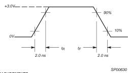
MEASUREMENTS: All circuit delays are measured at the +1.5V level of inputs and outputs, unless otherwise specified.
