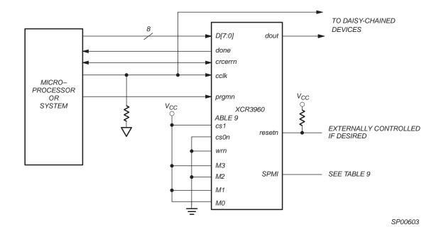
Figure 21: Synchronous Peripheral Configuration
