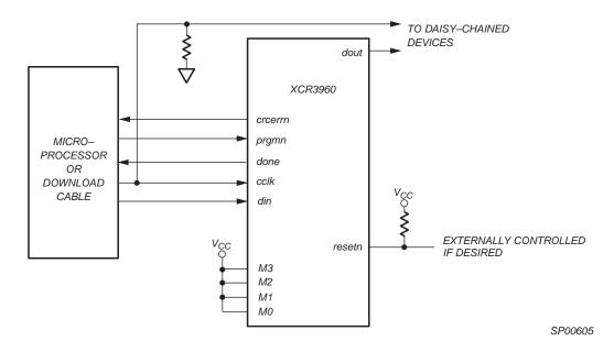
Figure 23: Slave Serial Configuration Schematic
