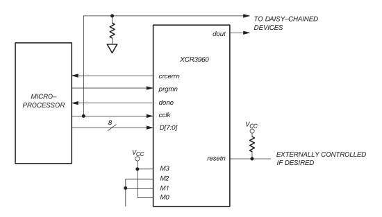
Figure 25: Slave Parallel Configuration Schematic
