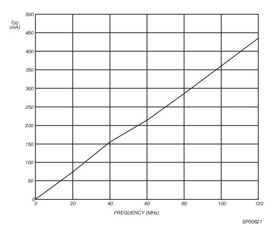
Figure 6: I<sub>CC</sub> vs. Frequency @ V<sub>CC</sub> = 3.3V, 25°C
