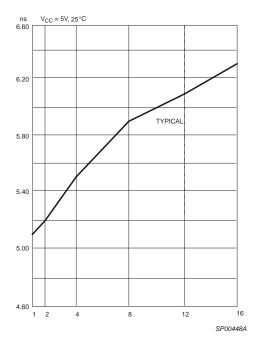
Figure 5: t<sub>PD PAL</sub> vs Outputs Switching
