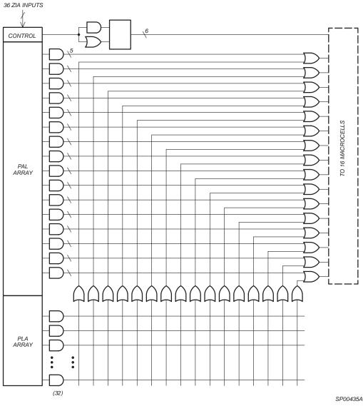
Figure 2: Xilinx XPLA Logic Block Architecture
