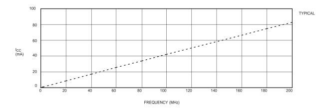
Figure 5: I<sub>CC</sub> vs. Frequency at V<sub>CC</sub> = 5V, 25°C
