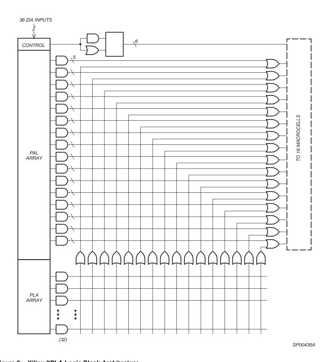
Figure 2: Xilinx XPLA Logic Block Architecture
