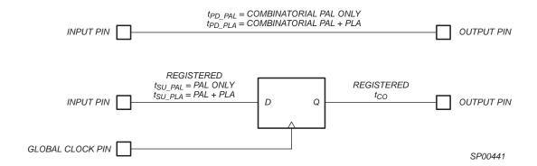
Figure 4: CoolRunner Timing Model
