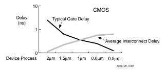
Figure 3: Relative Importance of Interconnect vs. Gate Delay
