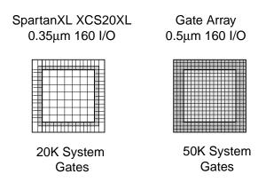
Figure 2: SpartanXL Device Matches
