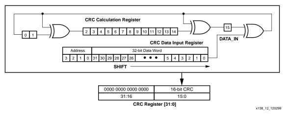
Figure 12: Serial 16-bit CRC Circuitry
