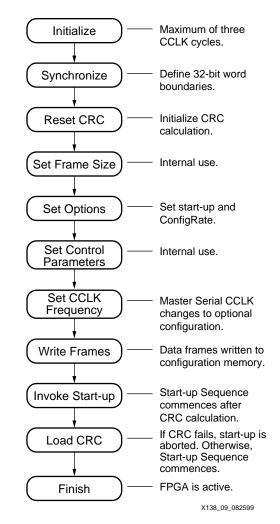
Figure 9: Internal Configuration Processing Flow
