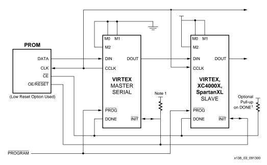
Figure 3: Master/Slave Serial Mode Circuit Diagram
