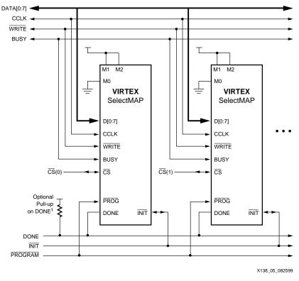
Figure 5: SelectMAP Mode Circuit Diagram
