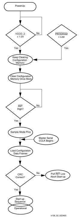
Figure 2: Configuration Flow Diagram
