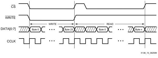
Figure 15: Readback Clocking Sequence
