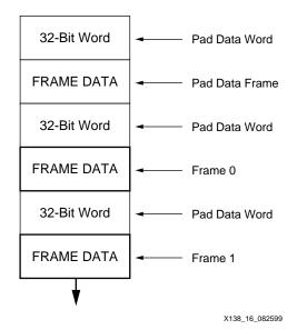
Figure 16: Readback Data Stream
