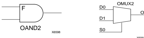
Figure 7: AND & MUX Symbols in Spartan-XL IOB
