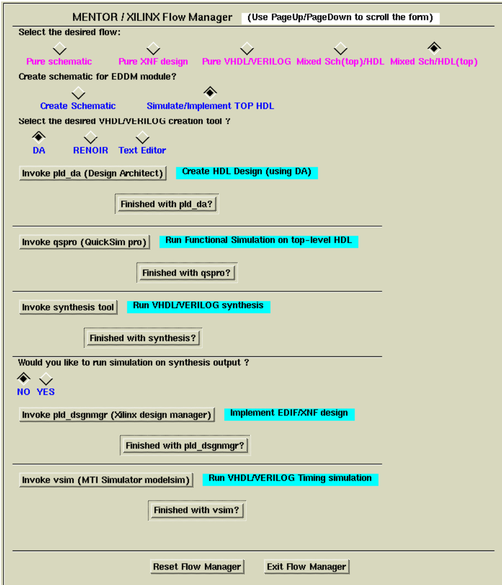
Figure 7-6 Mentor/Xilinx Design Manager Mixed Sch/HDL(top) — Simulate/Implement Top HDL Mode
