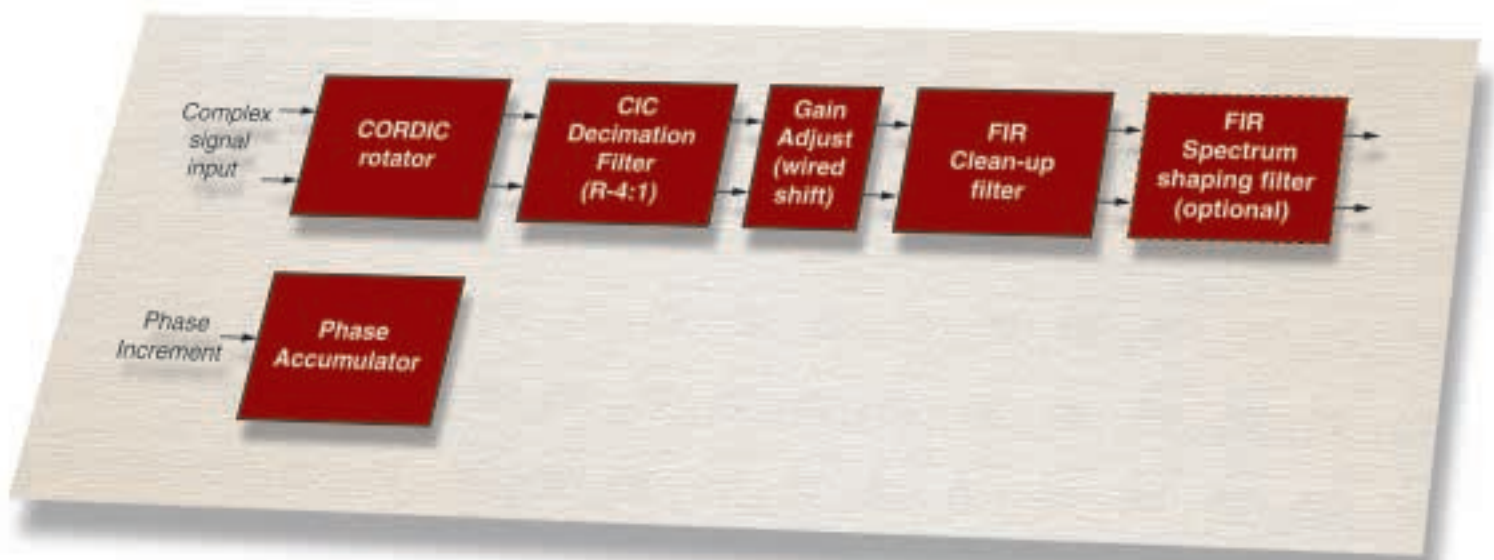
Figure 2-FPGA implementation of a digital down converter
