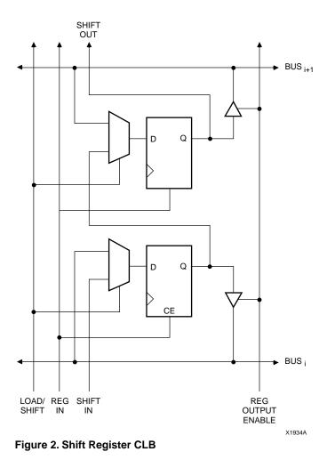
select data. For loading, data is taken from the bus; for shifting, it is taken from the adjacent flip-flop. A register enable is also provided, that must be asserted for either loading or shifting the register.
