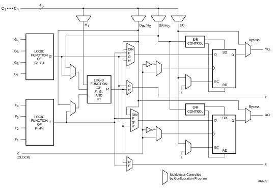
Note: The function generators and registers can be used together or independently. Dedicated carry logic is not shown.
