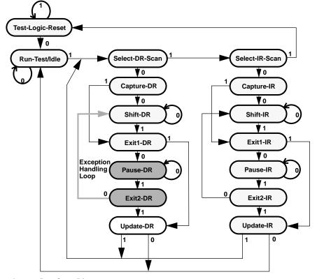
Figure 2: Test Access Port State Diagram
