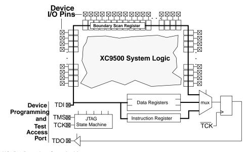
Figure 1: XC9500 Boundary Scan Architecture
