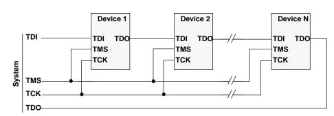
Figure 2: Single Port Serial Boundary-Scan Chain
