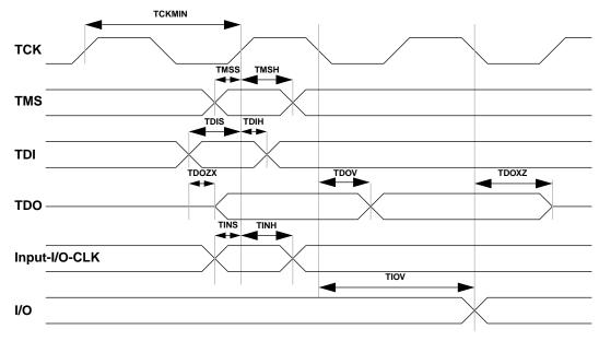
Figure 1: Test Access Port Timing
