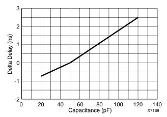
Figure 5: Additional Delay at Various Capactive Loads
