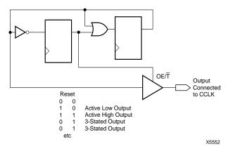
Figure 3: Additional CCLK-Pulse Generator
