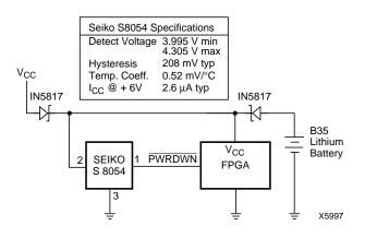
Figure 1: Battery Back-up Circuit
