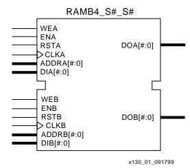
Figure 1: Dual-Port Block SelectRAM+ Memory
