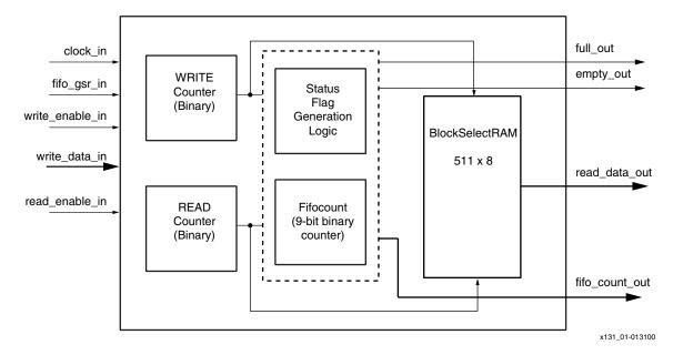
Figure 1: 511 x 8 Synchronous FIFO
