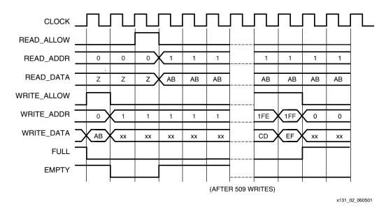
Figure 2: 511 x 8 Synchronous FIFO
