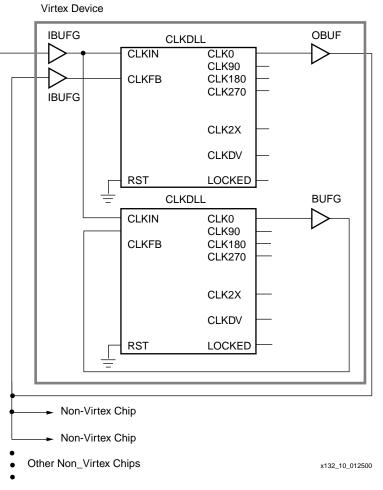
Figure 10: DLL De-skew of Board Level Clock
