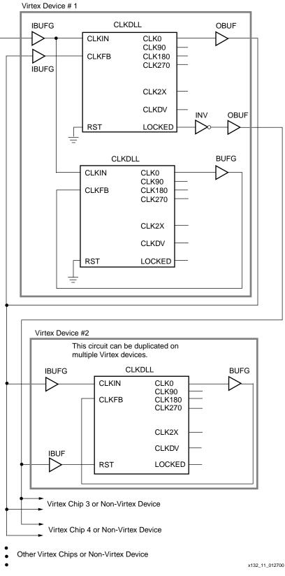
Figure 11: DLL De-skew of Board Level Clock
