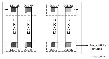
Figure 15: DLLs in Virtex-E and Virtex-EM Devices
