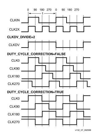
Figure 7: DLL Output Characteristics
