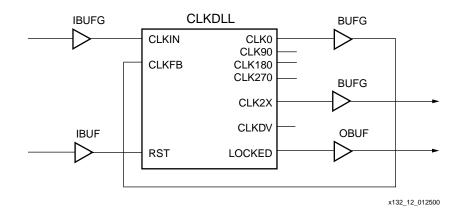
Figure 12: DLL De-skew of Clock and 2x Multiple
