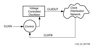
Figure 2: Phase-Locked Loop Block Diagram
